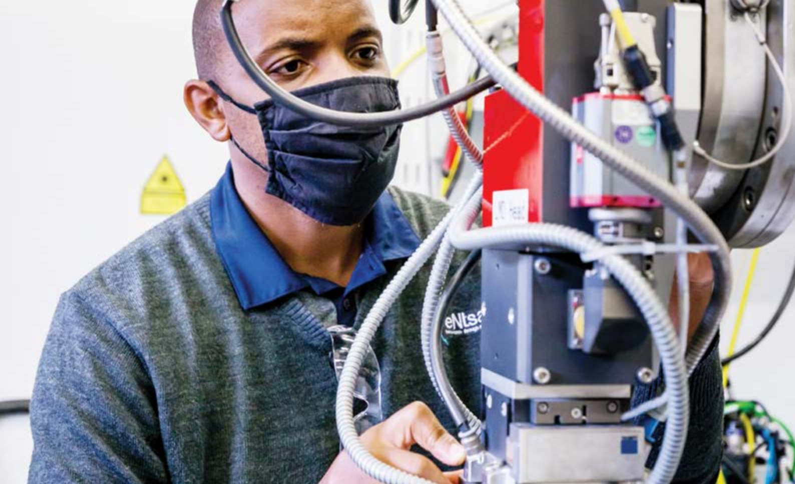
Dr Davies Tsikayi replaces the laser metal deposition head on the laser for research at eNtisa
