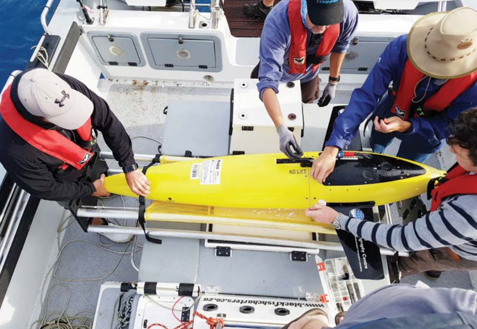
Ocean gliders are used to survey and gather data from the oceans
