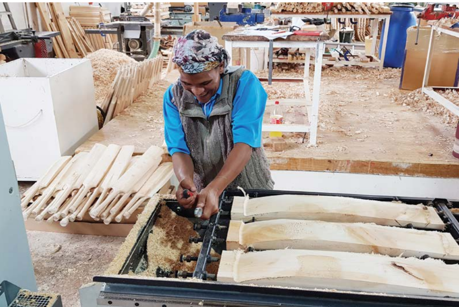
eNtsa worked with cricket bat manufacturer Bellingham and Smith to develop a wood router to speed up production
