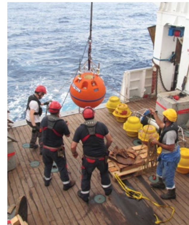
ADCP (Acoustic Doppler Current profiler) mooring being deployed at MADRidge to collect data on ocean currents, temperature and salinity. Photo courtesy Prof Mike Roberts
