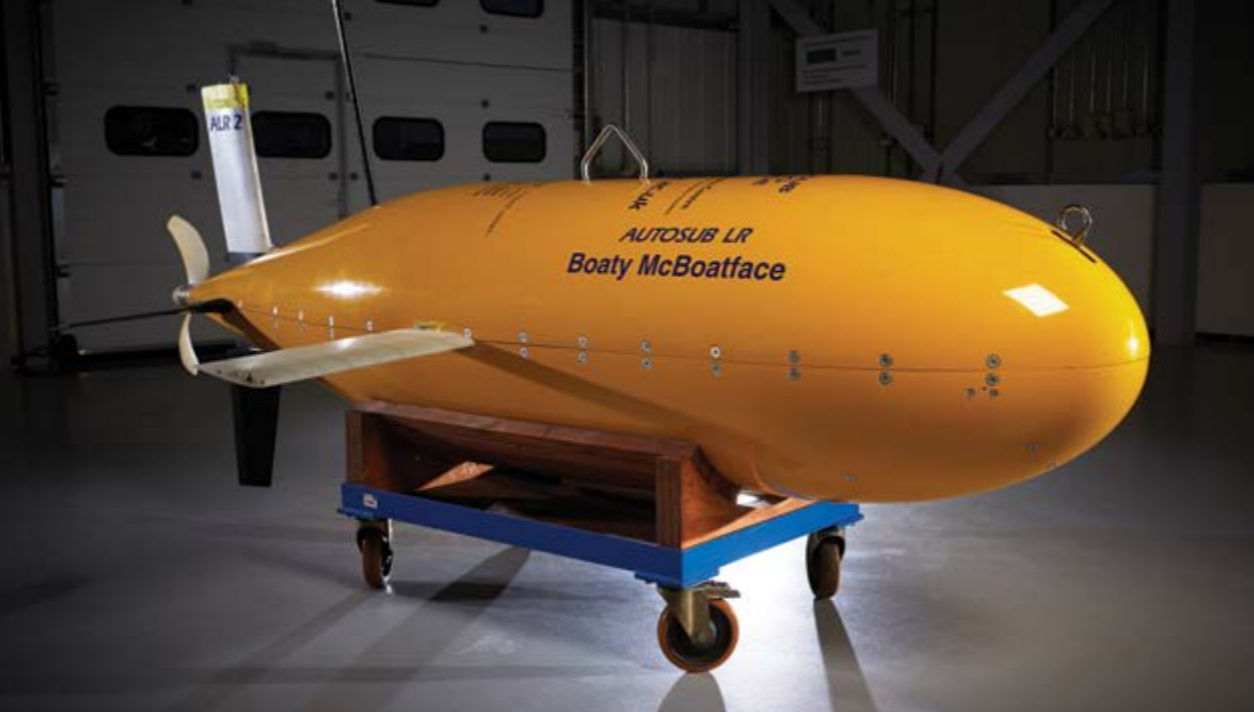
Boaty McBoatface – one of the National Oceanography Centre's autosubs – a long range autonomous vehicle that can travel for many kilometres and to great depths underwater, gathering scientific data. Photo: National Oceanography Centre (NOC)
