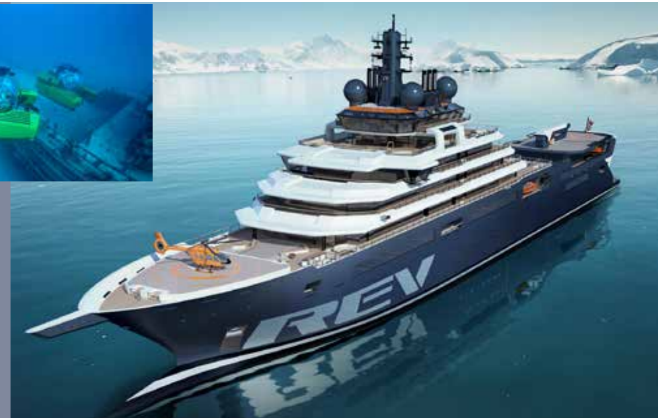
Top – Triton: a three-person ocean research vessel with a diving depth of 2300m that will be used by researchers on REV I. Bottom – Rendering of REV I, the largest, most advanced marine research platform in the world, currently being built in Norway, will help the world to better understand our oceans and what is happening to our marine resources. Photos: REV Ocean
